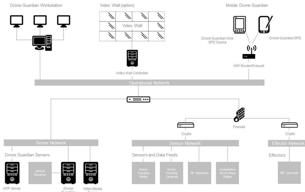
Figure 2: L3 Drone Guardian Network Architecture
