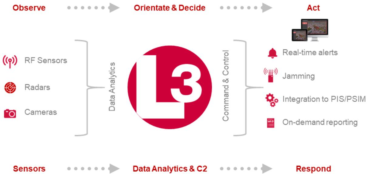
Figure 1: L3 Drone Guardian Effects Based Defence OODA Cycle
